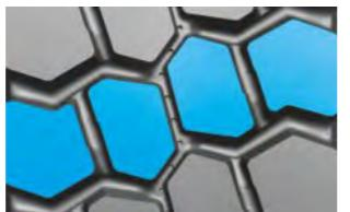
Integrated tie bars prevents stone drilling and guarantee longer mileage
