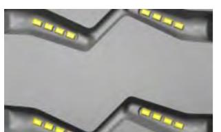
Stone ejector platforms prevent tread damage from stone drilling
