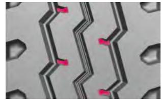
Heavy siping provides good braking stability and high lateral traction on wet and dry surface
