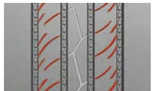
Shoulder heat dissipation design reduce tread rigidity and improve the durability of tyre
